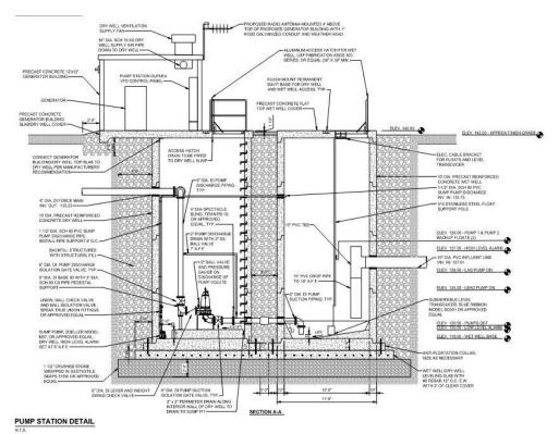
Figure 7: Wet Well/Dry Well Pump Station
